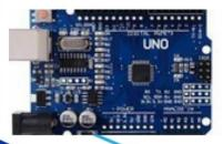
Arduino consists of both a physical programmable circuit board (often referred to as a microcontroller) and a piece of software, or IDE (Integrated Development Environment) that runs on your computer, used to write and upload computer code to the physical board.
